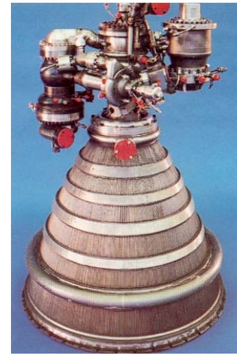
Space Engine \text{LH}_2/\text{LOX} = 1 : 6 I_{\text{sp}} = 473 \text{ s}
