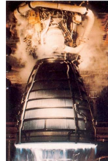
Space Shuttle \text{LH}_2/\text{LOX} = 1 : 6 I_{\text{sp}} = 455 \text{ s}
