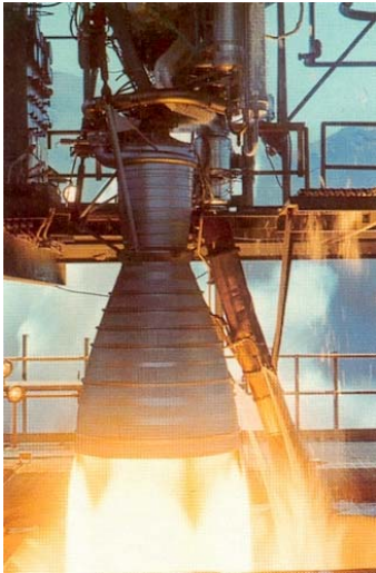
RS-27, Delta \text{HC/LOX} = 1 : 2 I_{\text{sp}} = 262 \text{ s}
