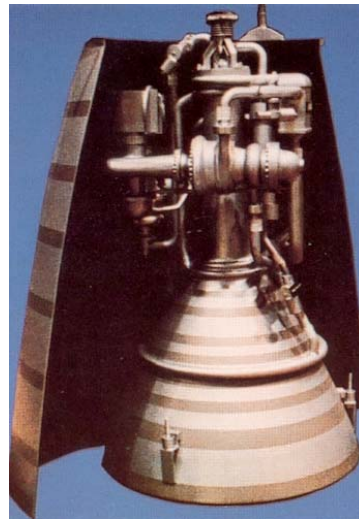
RS-44 \text{LH}_2/\text{LOX} = 1 : 6 I_{\text{sp}} = 480 \text{ s}
